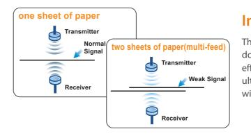
The ultrasonic sensor detects double feeding of original documents during scanning, and prevents double feeding and effectively scans documents of different weights or thickness. The ultrasonic function can be turned off when scanning document with labels, sticky notes, or taped receipts.
